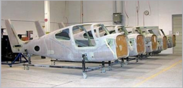
Fuselages ready to have landing gear and wings installed
