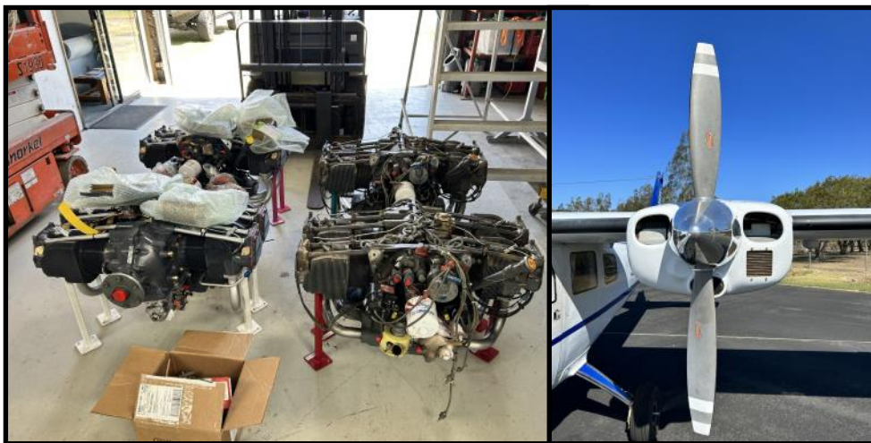
The new engines ready for installation (left) and installed (right)
